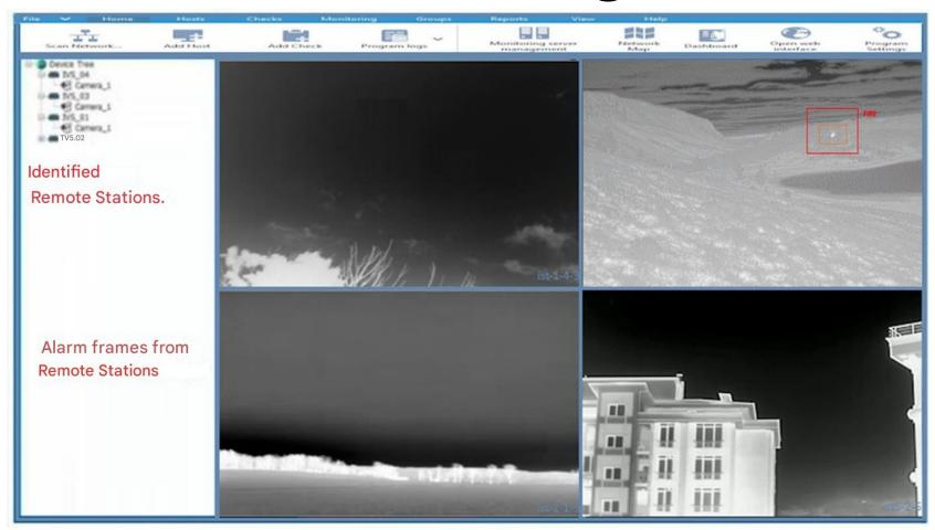
If an alarm is detected in the system at a station, smoke, fire, moving object, etc., it sends a picture, short video and coordinates and a time stamp to the central monitoring system. The last image appears on the central viewing screen.
